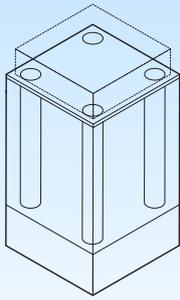
TTT Deep Pile Foundations are designed for sites where a competent bearing stratum, at least 3.0m thick, is identified below ground (as per MBIE Guidance 2012, section 15.2.2, p. 15.7).
