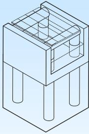
TTT Bridges can be specifically designed for many applications, including residential access ways, pedestrian bridges, cycle bridges, highway bridges, and more. The foundations of TTT Bridges are similar to TTT Deep Pile Foundations and likewise use TTT MultiPole SED piles. These are combined with TTT MultiPole UniLog bearers for strength, durability, and easy installation.
